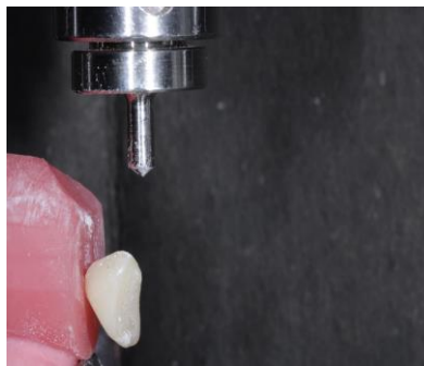
Figure 1. Shear Bond Strength Analysis of the Sample after Fracture
