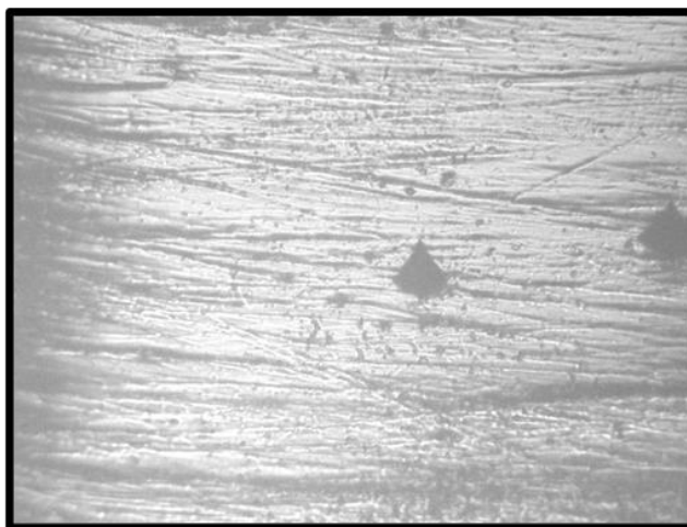
Figure 4. Vicker's Hardness Test
